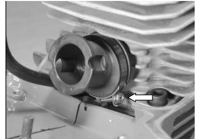
13.5 Remove cylinder screws (4) and wave washers.
